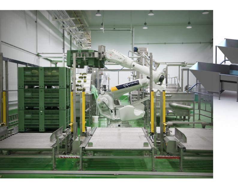
Anthropomorphic robots can be programmed to handle any element. Therefore, Gémina designs and creates solutions adapted to the different costumer's needs. Gémina also creates different solutions for different containers: metallic or plastic drums, pallets, boxes, cans, bags, packs, etc.
